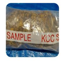
Final Sample a. 3 x 500g or b. 4 x 500g c. Sealed and labelled d. Sent to KSS
