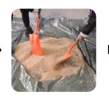
Aggregate Sample a. Min 4kg b. Mix, cone, quarter, reject opposite quarters
